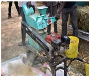
Processing animal feed from invasive species ( Prosopis juliflora ) and acacia . The machine can also be used to process hay.
