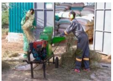
Processing animal feed from invasive species ( Prosopis juliflora ) and acacia . The machine can also be used to process hay.
