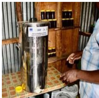
A honey warmer, preventing crystallisation of the honey, at the honey aggregation centre
