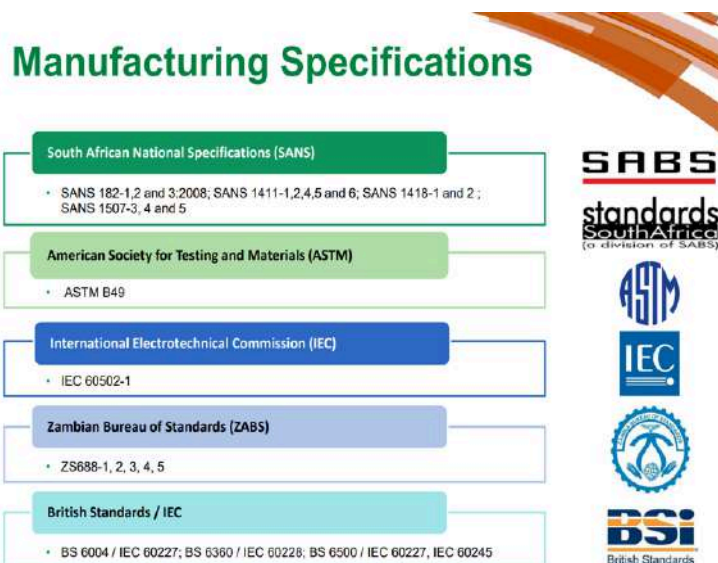
Figure 12 - Domestic, Regional and International Manufacturing Specifications and Standards for Wire & Cable Manufacturers
